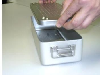
2. Use a small object (e.g. a screwdriver) to remove the seal from the lid groove and slide out the seal.
