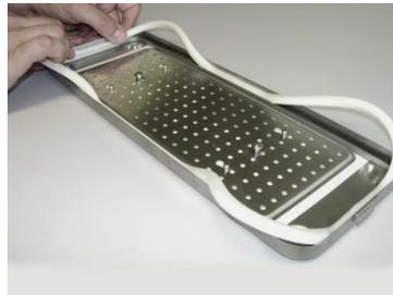
Make sure not to twist the seal when inserting it!
